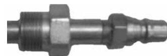
KJ1044B Tank Fill Stem – For use with the KJ1000 Nitrogen Intensifier and the KJ1043 Nitrogen Discharge Hose. The tank fill stem allows consolidation of low pressure nitrogen bottles into one tank at pressures from 0 to 5500 PSI.
